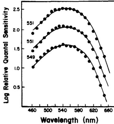
Fig. 1. Flicker photometric spectral sensitivity functions obtained from three *Cebus* monkeys. These animals have one of the two types of dichromacy found in this species. The solid circles are sensitivity values obtained by equating the effectiveness of monochromatic test lights and an achromatic reference light. The solid lines are the best fitting visual pigment nomograms, the spectral peak of which is given on each function. The curves are arbitrarily positioned on the sensitivity axis.
